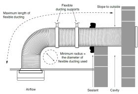
Where flexible ducting is used the diameter must be maintained and it is good ventilation practice that the ducting is extended to 90% of its possible length in order to maintain the best possible airflow. Ensure that flexible duct connections are not over tightened to the fan outlet spigot. To maximise airflow rigid ducting should be used. The fan and ducting should be installed in accordance with the requirements of the Domestic Ventilation Compliance Guide, part of the Building Regulations.
